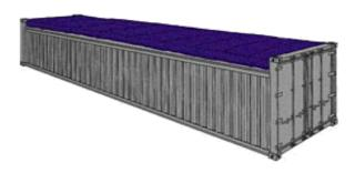
For large and/or high pieces that can not be loaded through container doors, such as machineries, marble, glass sheets, etc
